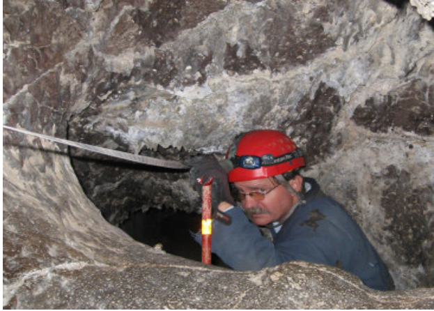
Jim Wolf pulls tape surveying in Sentinel Cave in Lava Beds National Monument. The strong and variable magnetic field in the 36,000 year-old basalt of Mammoth Crater effects magnetic compasses so much that the compasses must be perched atop 0.3 meter long wooden dowels.
