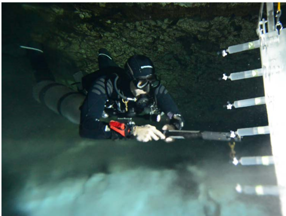
Figure 1. Research in an anchialine cave: obtaining physicochemical profiles above the halocline (blurry water bottom of the picture). Diver: David Brankovits. Photo: Rogelio Mier.
